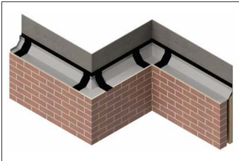
Figure 6 Trays, Corners, and Stop ends over sealed with DAFA Moisture Barrier Tape
